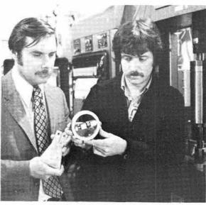
TEST CHAMBER IN AREA 8 is used to subject materials samples to hydrogen under high pressures and temperatures. Jim Swisher (8313), left, and Anton West (8314) examine steel ring which has also undergone stress during hydrogen exposure.
